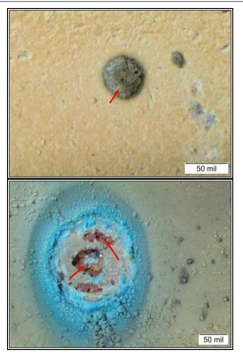
**Figure 6:** Photomacrographs showing the ID of a pipe exhibiting a tubercle (top, arrows) and the pitting (bottom, arrows)
