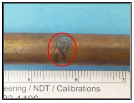
Figure 3: Photograph of an as-received pipe showing leak location (encircled)
