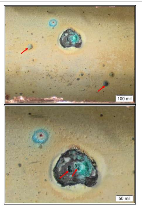
**Figure 5:** Photomacrographs showing the ID of a pipe exhibiting tubercles (top, arrows) and the pitting (bottom, arrows)
