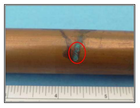
Figure 2: Photograph of an as-received pipe showing leak location (encircled)
