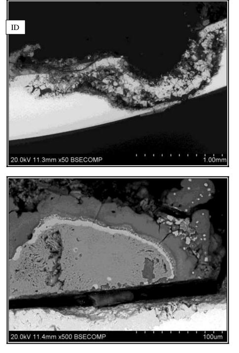
**Figure 11:** Back-scattered electron image of a pipe sample exhibiting localized pitting corrosion (top), and the OD deposit (bottom)
