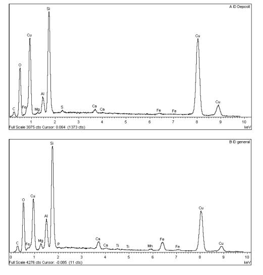
Figure 8: EDS spectra of the ID deposits from different pipes
