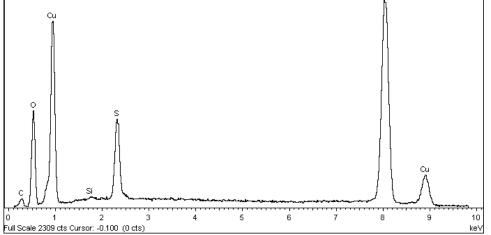
**Figure 7:** Back-scattered electron image (top) and EDS spectrum (bottom) of a corrosion pit (bottom)
