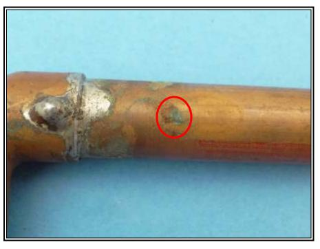
Figure 1: Photograph of an as-received pipe showing leak location (encircled)
