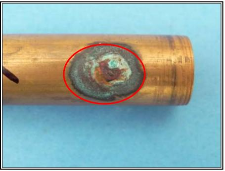
Figure 4: Photograph of an as-received pipe showing leak location (encircled)
