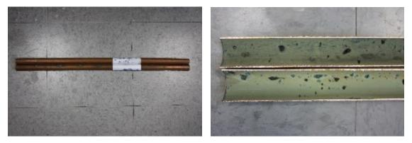
Figure A.8 – Pipe #8 exterior (left) and interior surface (right)
