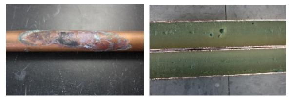
Figure A.4 – Pipe #4 exterior (left) and interior surface (right)
