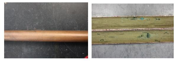
Figure A.5 – Pipe #5 exterior (left) and interior surface (right)
