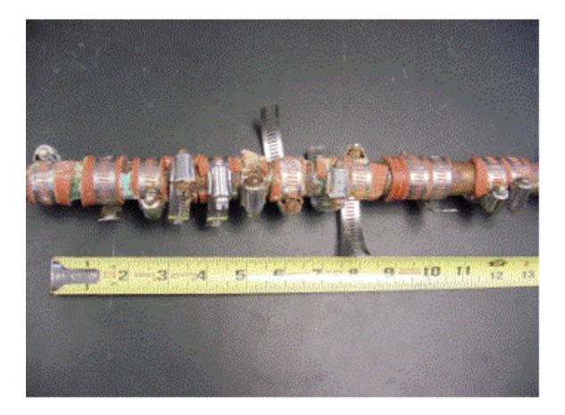
Figure 9: Pipe from Arlington, Virginia Water System with Clamps to Stop Pinhole Leaks (Courtesy Dr. Marc Edwards)
